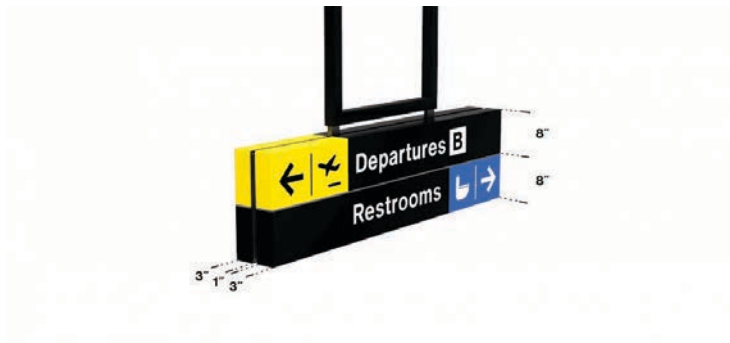
Sign box showing typical dimensions.
