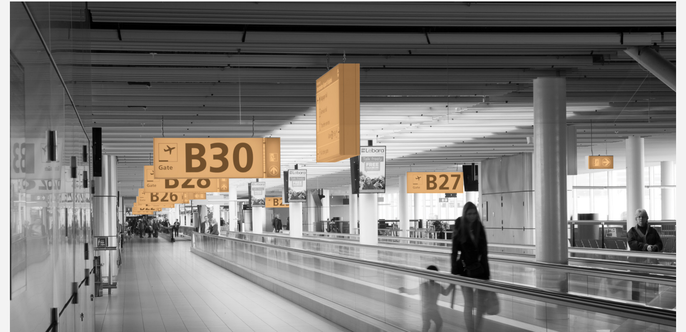
The wayfinding zone is placed directly above the flow zone. This keeps wayfinding always in passengers' optimal field of view and free of visual distractions.
