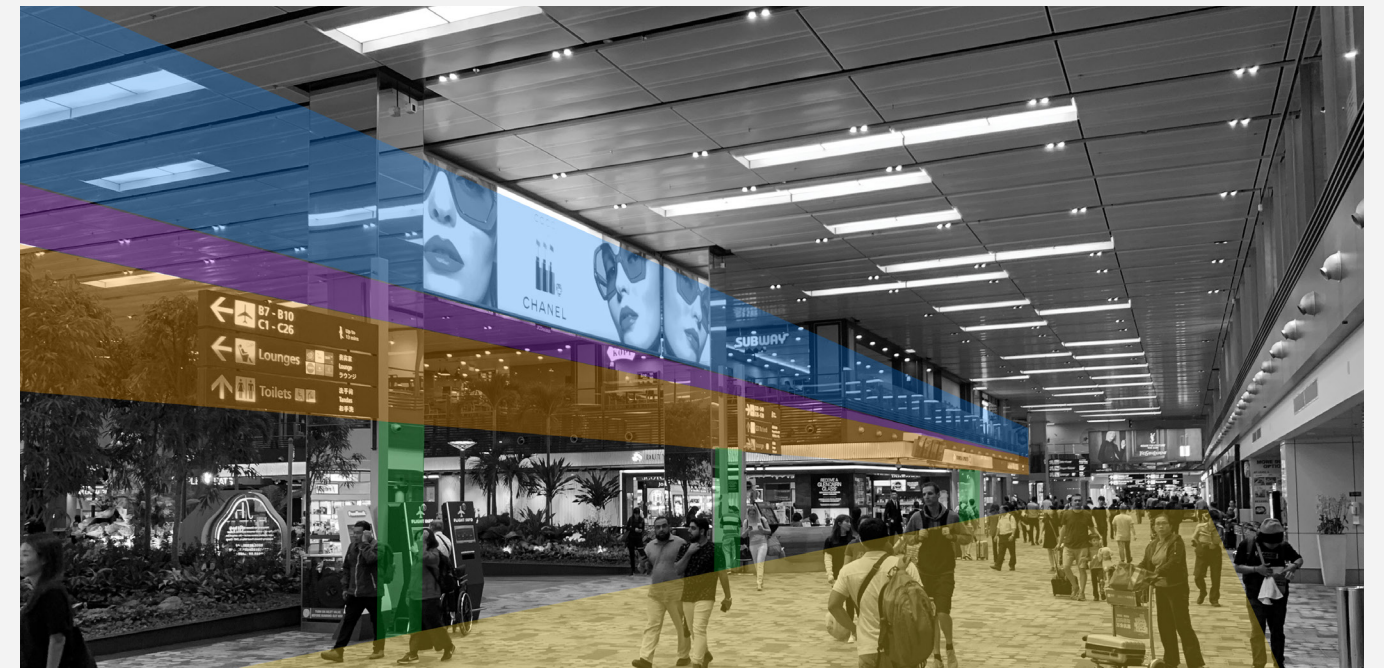
The wayfinding zone is clearly separated from commercial media by a buffer zone. A designated space for each media type reduces competition and allows passengers to digest both types of media.
